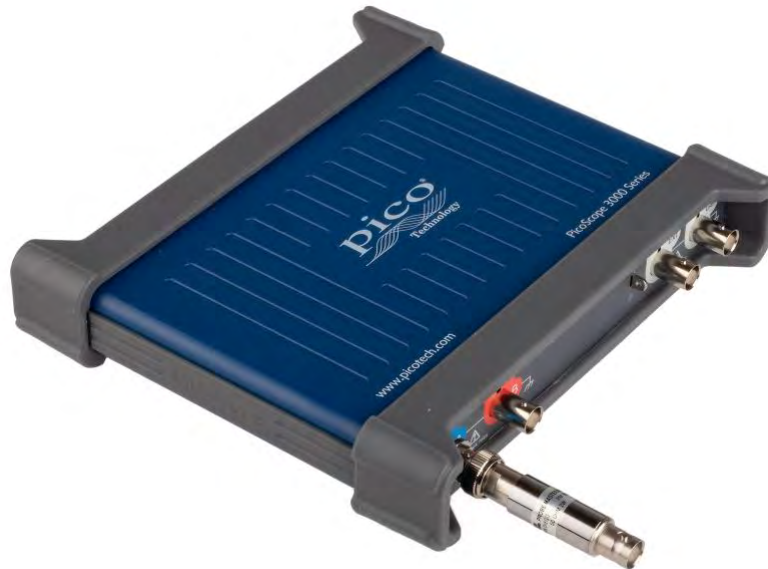
Figure 4: Oscilloscope used to identify sweet spots and verify EM glitches
