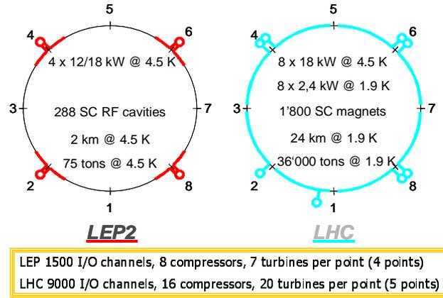
Figure 2: LEP2 and LHC simplified layouts
