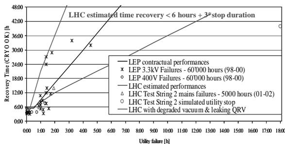
Figure 4: Mains failure recovery performances.
