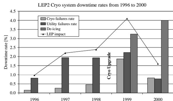
Figure 2: cryogenic downtime impact on LEP machine
