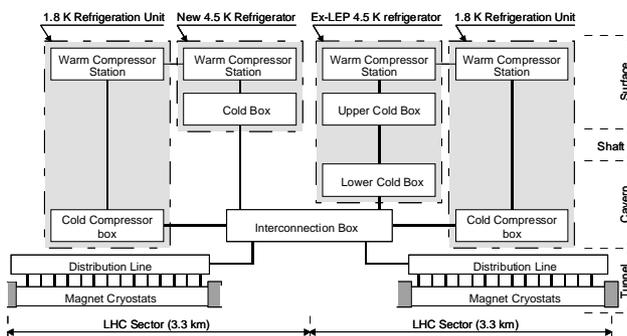
Figure 3: The cryogenic system architecture per point.
