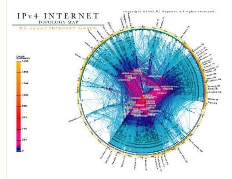
The map shows a snapshot of the major "choke" points, or "core carriers," for Internet traffic as it exists today. There are not that many choke points—think of these as "hubs" in a hub and spoke airline network. (The choke points are in the magenta area in the middle of the diagram.)
