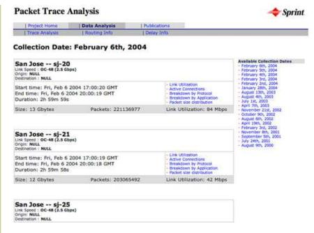
Notice anything interesting here? Link utilization for these links is minimal. These OC48 links can support upto 2.5 gigabits/sec but the utilization is barely more than 100megabits persecond. And the storage needed for these traces is minimal as well.
