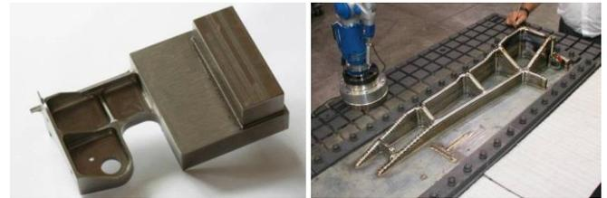
Fig. 35 – Sample advanced titanium fabrication processes. Left: Rough-machined titanium linear friction welded 787 floor beam fitting prototype. Right: Titanium additive manufacturing 787 side frame demonstration article.
