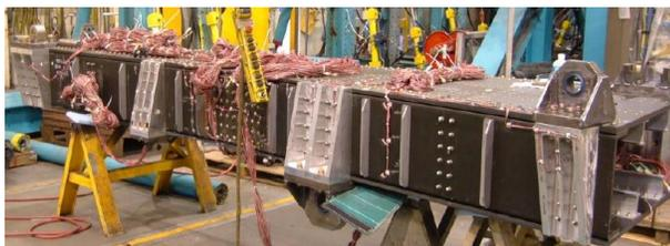
Fig. 31 – Subcomponent testing example: Co-bonded Boeing 787 composite “mini box” test article with VID.
