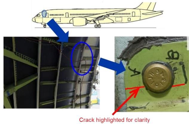
Fig. 18 – Example of a 787 full-scale fatigue test crack finding. Cracked fuselage door surround intercostal clips, found at the 72,000-flight inspection. In this case, the corrective action was to remove and replace the cracked parts.
