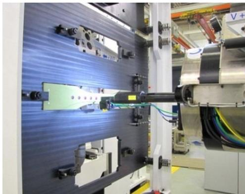
Fig. 38 – Fatigue test specimen being assembled in a production 737 PAL gantry system.
