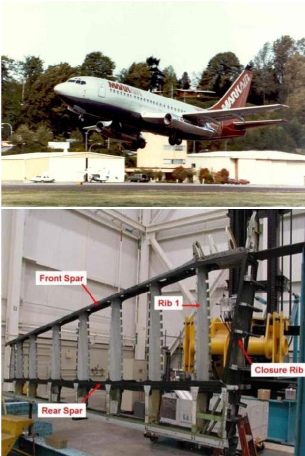
Fig. 23 – Boeing 737 composite horizontal stabilizer technology demonstrator.
