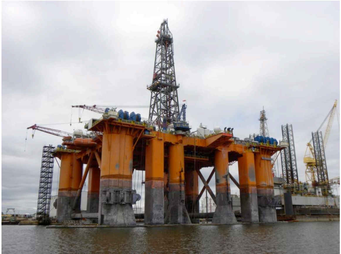
THE NOBLE DRILLER – A SEMI-SUBMERSIBLE DRILLING RIG
