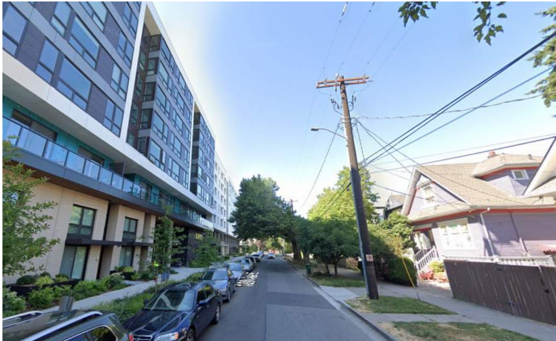
Ground level change in cladding and fenestration at transition of zones.
