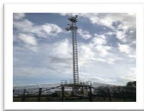
**Remote Video Surveillance Systems (RVSS)**, provide persistent, wide-area surveillance and real-time video analytics of rural, urban, and remote areas. Each unit consists of color and infrared cameras mounted on fixed or relocatable towers, or on building structures, and remotely operated from Border Patrol stations.
