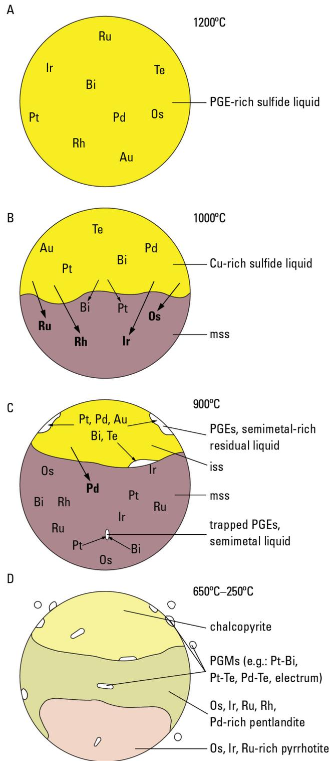
**Figure 8.** Schematic representation of a fractionating, platinum-group elements (PGE) enriched immiscible sulfide liquid droplet. Major partitioning behavior at each stage is emphasized by bold text. (A) Immiscible sulfide liquid. (B) Crystallization of monosulfide solid solution (mss). Os, Ir, Ru, and Rh partition into the mss phase. (C) Crystallization of intermediate solid solution (iss) from
