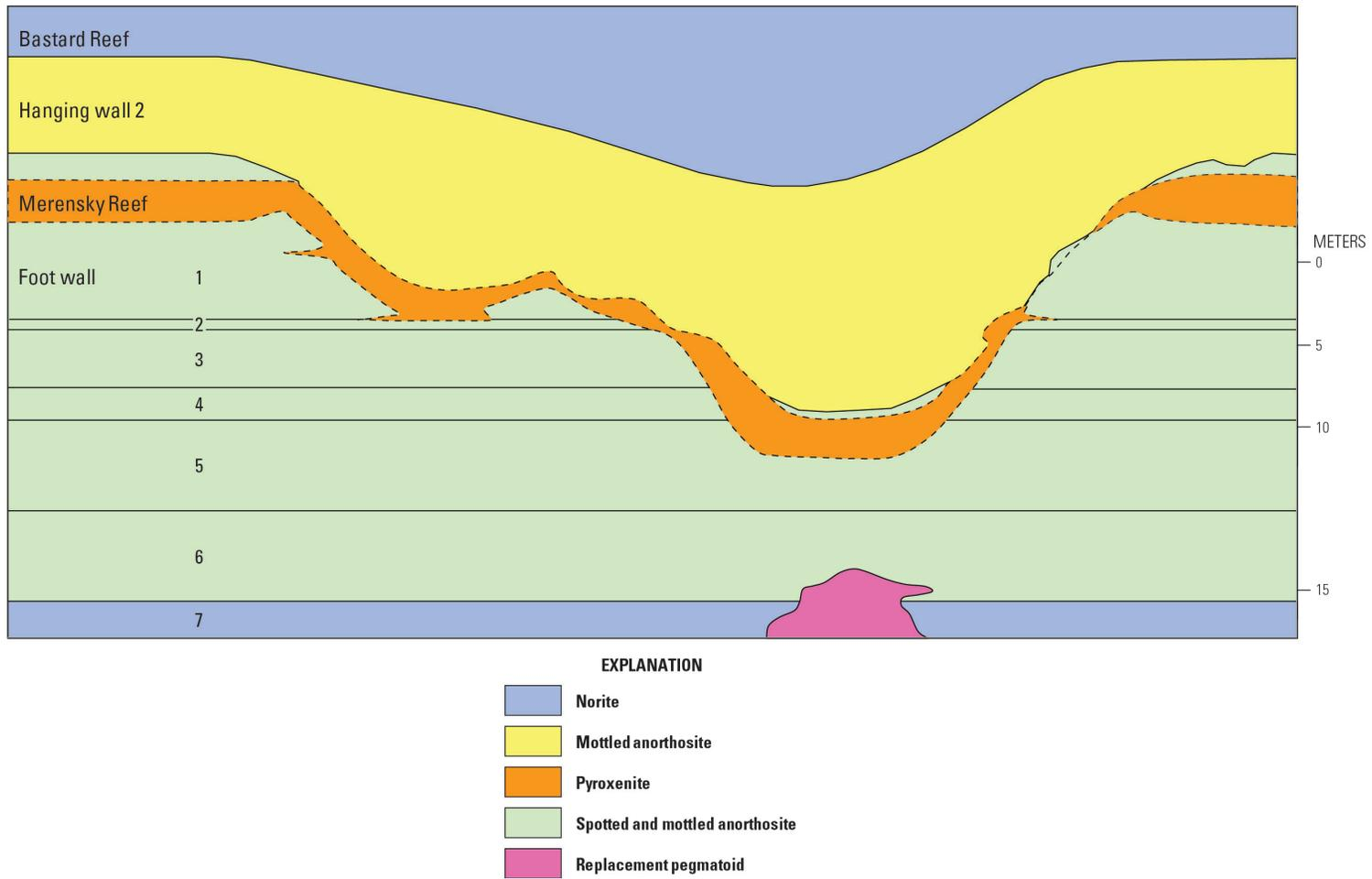
**Figure 7.** Section through two adjacent potholes illustrating the irregularity of the Merensky Reef, Bushveld Complex. Modified from Farquhar (1986).
