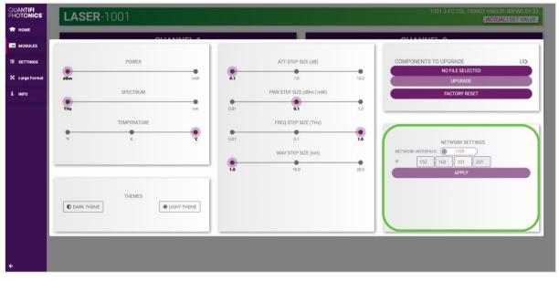
The value in the 3<sup>rd</sup> octet of the IP address can be changed to any available value. It is important to make sure that any other instruments connected to the computer do not share this new IP address, as there will be an addressing conflict.
