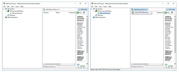
3. Select **Manual Entry of LAN Instrument**. Enter in the Hostname or IP Address. The top image is an example of operating remotely, the bottom image is an example of operating locally. Note when operating locally, enter in the localhost IP address of **127.0.0.1**. Click **Finish** to end the setup process.
