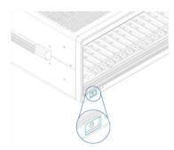
STEP 4: Push module into slot until resistance is felt from the backplane connection
