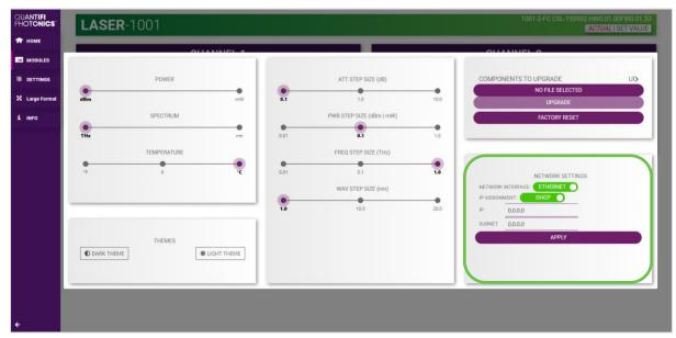
The addressing method can be changed to a static method, where the MATRIQ instrument will always have the same IP address over Ethernet. Typing in a **valid IP address and Subnet mask**, and then clicking **APPLY** will save the IP address into the settings of the instrument.
