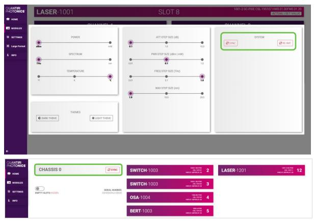
Clicking the **RE-INIT** button will bring up a prompt to continue, since this action will temporarily disconnect all modules while the re-initialization with the CohesionDriver service is in progress. Once it is complete, the page will be functional again.
