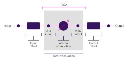
If some input and / or output offsets are specified, The VOA works as described in section 10.2. 10.2
