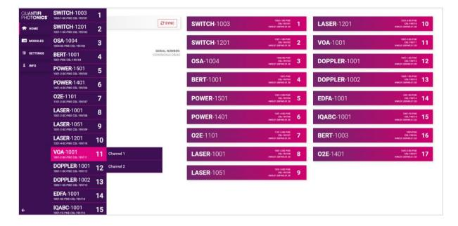
After clicking the desired VOA module, its control page is displayed. All information relating to the module such as model number, serial number and firmware versions are displayed in the top right corner of the window.
