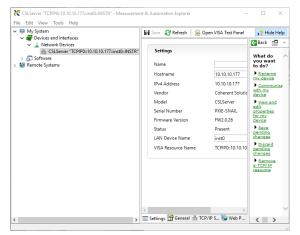
2. On the right-hand side panel, select **Open VISA Test Panel**. A new window will popup. Click the **Input / Output** button from the window menu.
