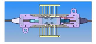
Figure 1(c). Silicon photonic VOA module with the cover removed
