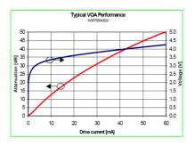
Figure 1(d). Measured VOA performance
