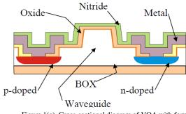
Figure 1(a). Cross-sectional diagram of VOA with forward biased p-i-n diode.
