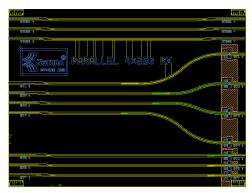
Figure 2(b): Mask layout of SiP Rx with Ge Detectors
