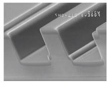
Figure 1(b) SEM view of mode transformer
