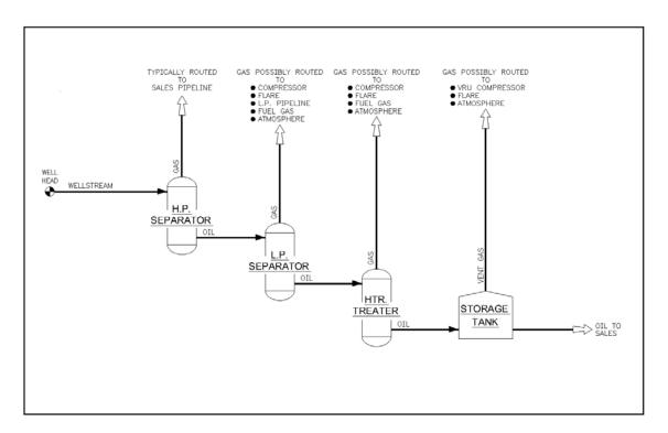
For each stage of flash (e.g., low-pressure separator oil to heater treater) that is vented to the atmosphere (locally or to remote vent) or flared (locally or to remote flare), the operator should give the following data:
