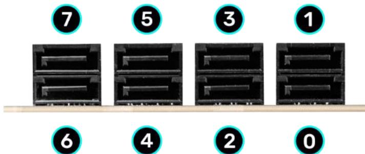
Intel® SATA ports on this platform natively support full AHCI and RAID functions. RAID mode supports RAID levels 0, 1, 5, and 10 through the Intel® controller, and all ports retain full AHCI functionality in RAID mode.
