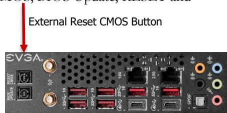
Use the Reset CMOS button to clear the BIOS before and after updating the BIOS, and as a troubleshooting option when the motherboard fails to POST (e.g. after installing new hardware, testing an unstable overclock, etc.).
