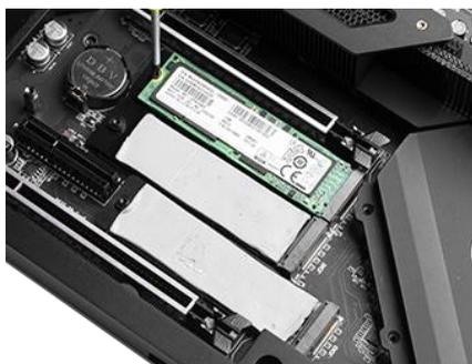
Please carefully check your M.2 devices for proper installation before moving on to the next step. If the M.2 device is not installed properly, the heatsink covers cannot be fully fastened.
