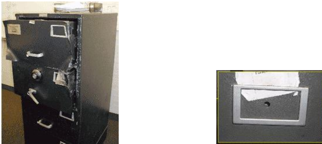
Figure 2: Compromises on GSA Security Containers
