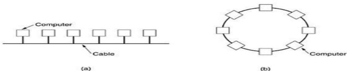
**Fig.1: Two broadcast networks . (a) Bus. (b) Ring.**
