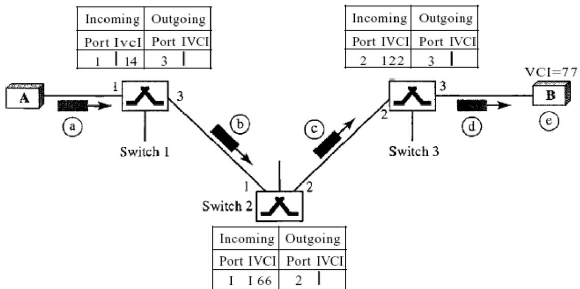
**Figure 4** Setup request in a virtual-circuit network
