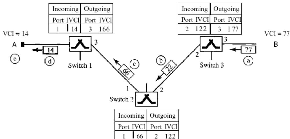
Figure 5 Setup acknowledgments in a virtual-circuit network
