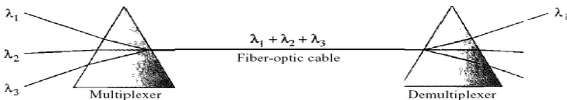
Figure 5 Prisms in wavelength-division multiplexing and demultiplexing
