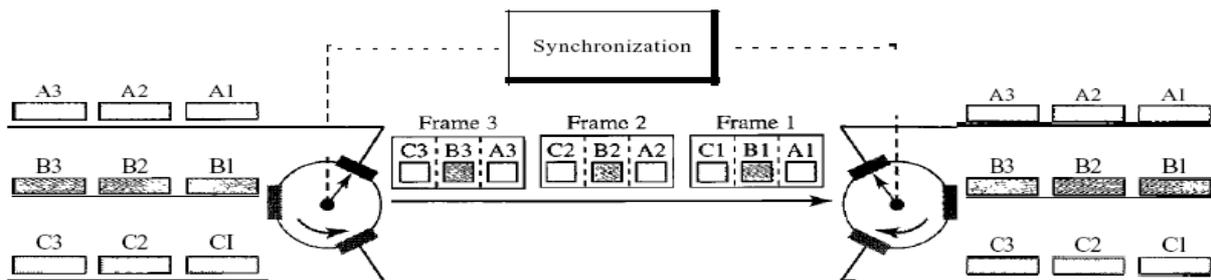
**Figure 8** *Interleaving*
