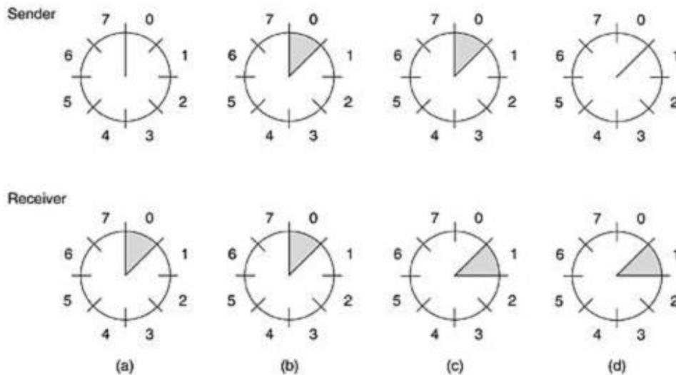
**Fig.8.A sliding window of size 1, with a 3-bit sequence number (a) Initially (b) After the first frame has been sent (c) After the first frame has been received (d) After the first acknowledgement has been received.**
