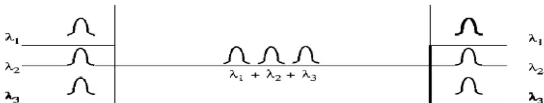
Figure 4 Wavelength-division multiplexing
